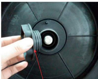
(1) Remove the spool retaining nut.
