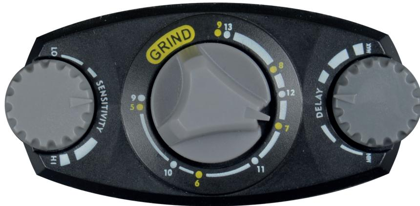
In grinding mode the darkening function is off. During this time the LCD is the brightest state, helping to get a clearer view next to a maximum protection.
